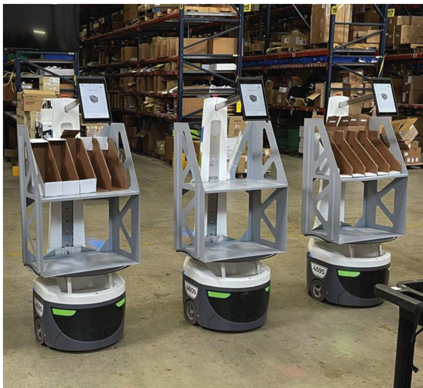
LocusBots minimize unproductive worker walking time and eliminate carrying or pushing carts by autonomously traveling to worker and pick locations.
